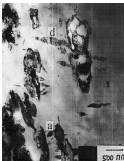
Figure 11 Photographs of the initiation, propagation, and termination of crazes in PVC/ABS blends: (a) initiation of crazes from the edge of one ABS particle and its termination at the edge of another ABS particle, (b) diffraction in the propagation of the crazes, (c) the uniform and integral network inside of the crazes formed in propagation, and (d) a combination structure of a whole craze and a fractured craze.
